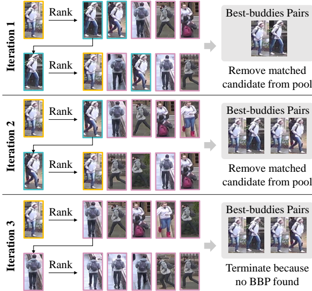
Fig. 2: Iterative best-buddies search algorithm. Images in yellow bounding boxes denote the query image. Images in green have the same ID as the query, while images in purple have different IDs. Note that our searching algorithm identifies positive image pairs based on the travelling patterns observed from unlabeled pedestrian data.
