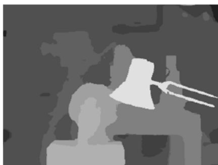
(c) weighted median filtering of (a) 134ms , Err. 1.66
