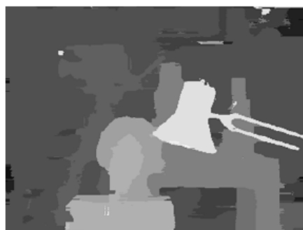
(b) guided agg. + LR check + hole-filling 246ms, Err. 2.08
