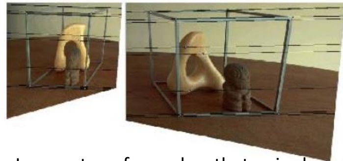
Images transformed so that epipolar lines are parallel.
