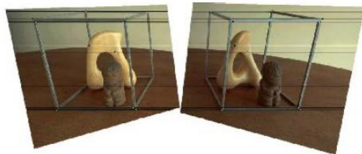
Final rectification that minimizes horizontal distortions. (Shearing)
