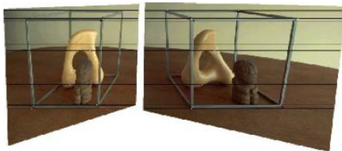
Images rectified so that epipolar lines are horizontal and aligned in vertical.
