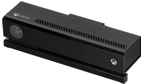
Kinect V2 (time of flight)
